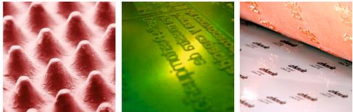
High resolution measurement at 43'000 ppi for high resolution imaging at 4'000 ppi to print gravure quality in flexo with high screen rulings and excellent solid ink laydown.
